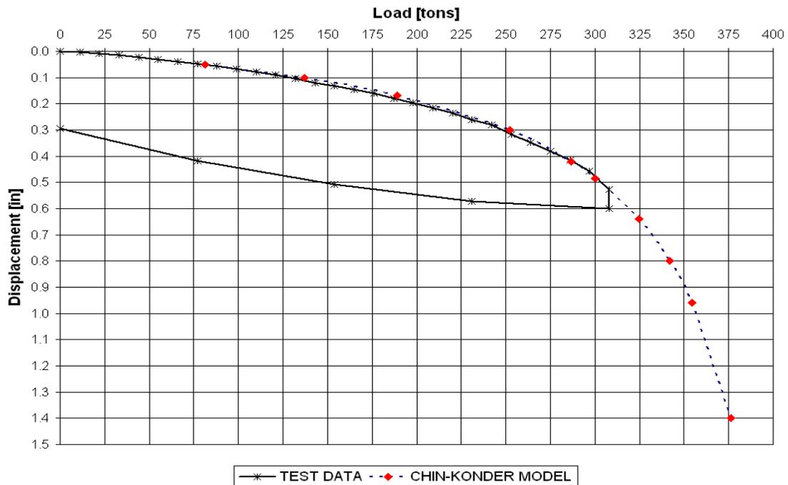
**Figure 10 – Applied Load vs. Pile Head Displacement**
