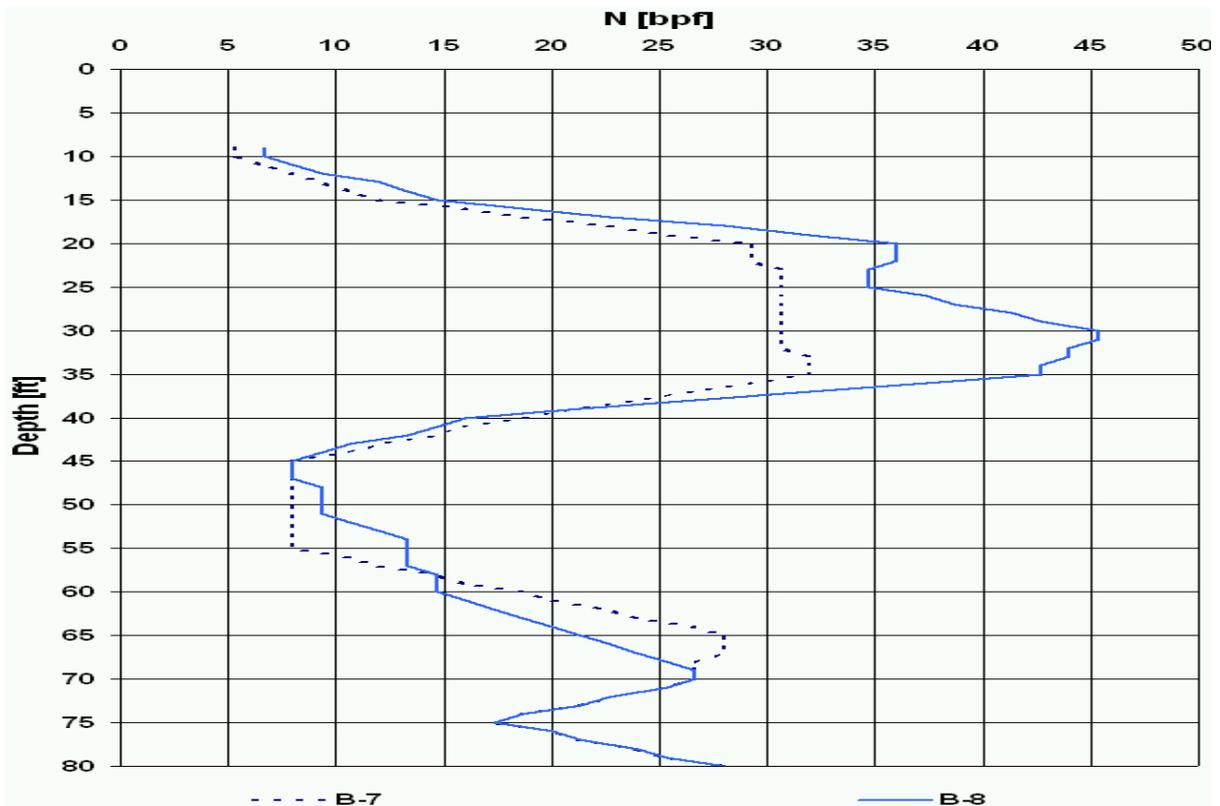
**Figure 14 – Composite Plot of SPT Results**
