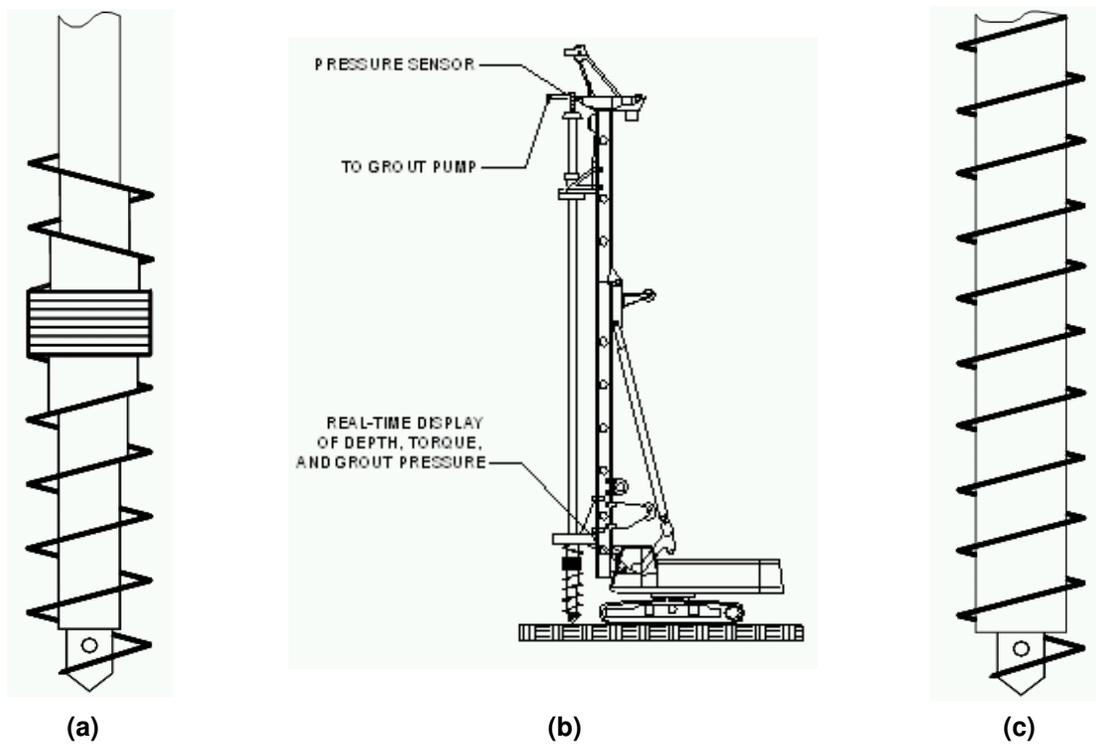
Figure 4 – Schematic of (a) Drilled Displacement Tool, (b) Drilling Platform and (c) Intermediate Displacement Tool
