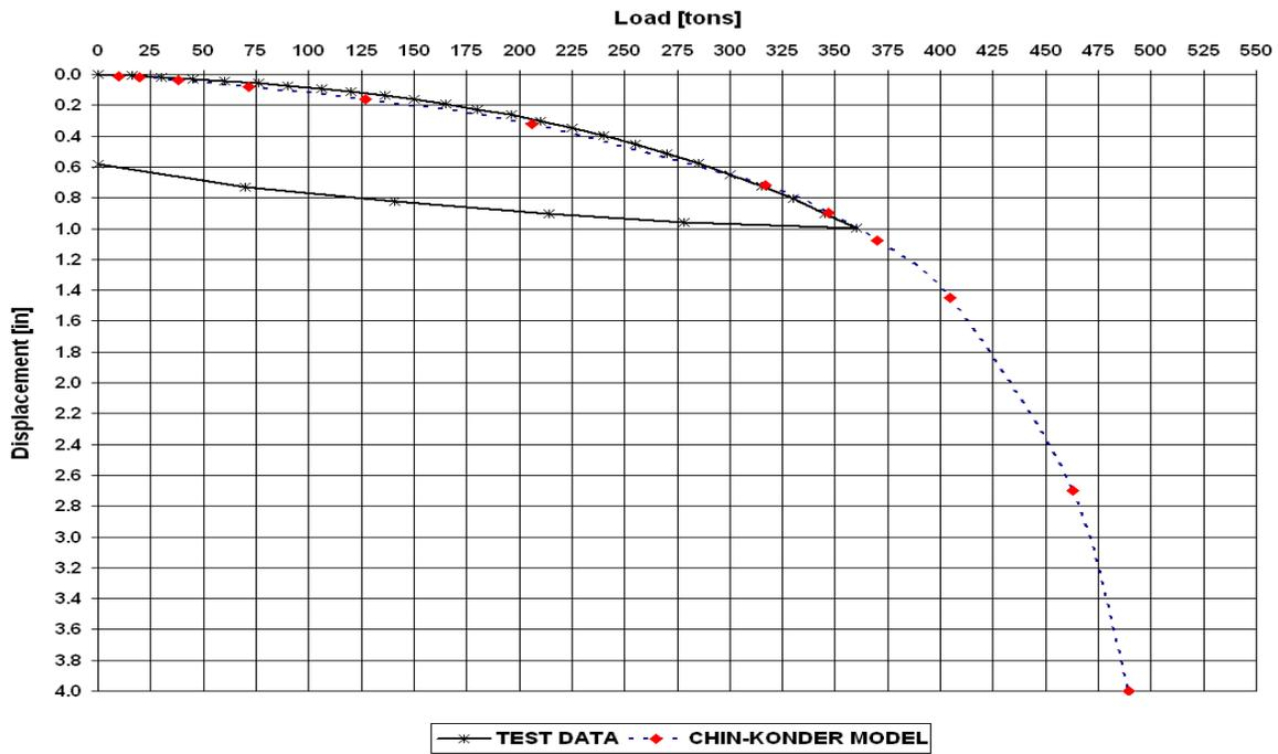
**Figure 12 – Applied Load vs. Pile Head Displacement**
