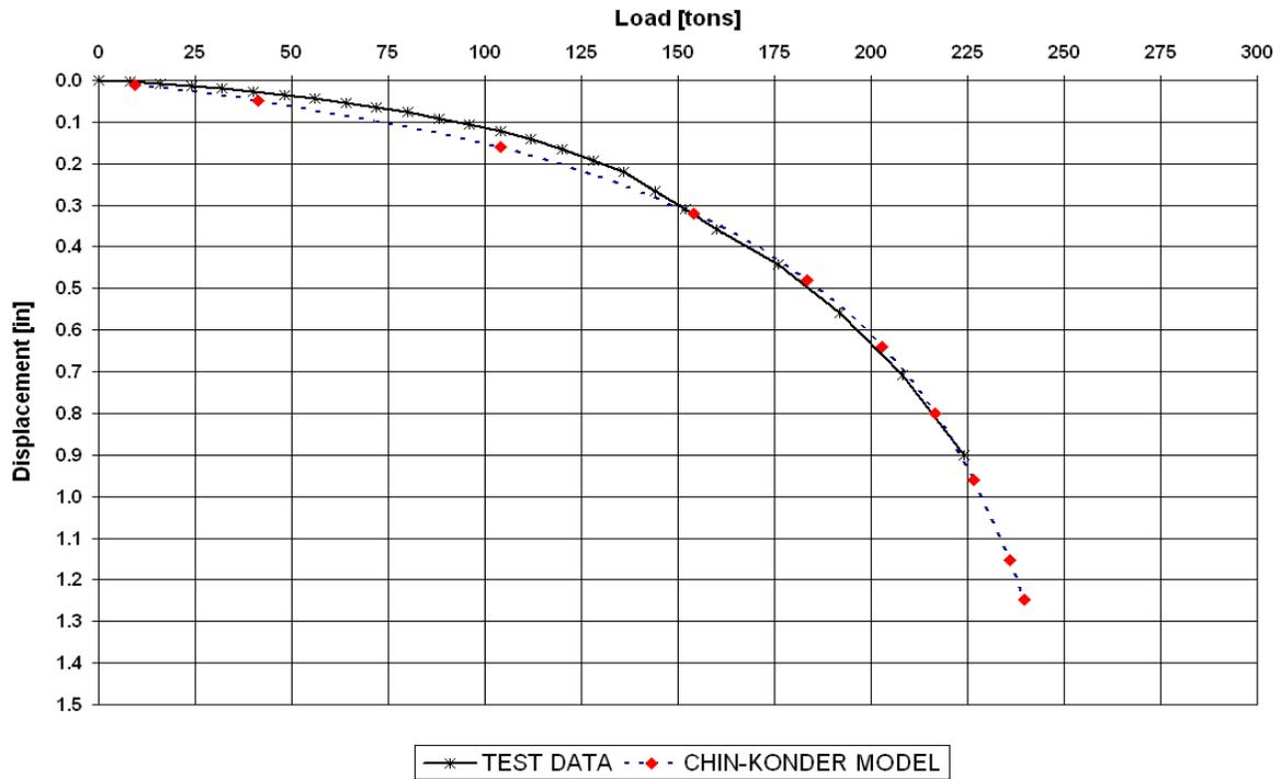
**Figure 17 – Applied Load vs. Pile Head Displacement**
