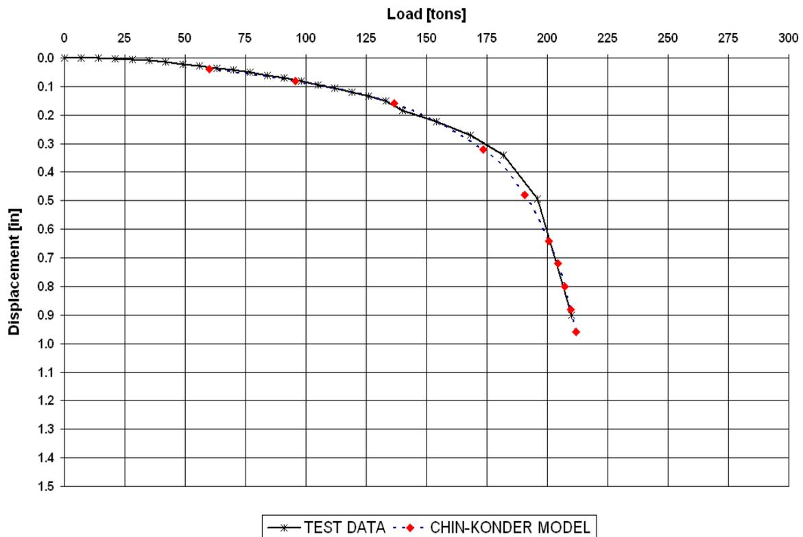
**Figure 19 – Applied Load vs. Pile Head Displacement**
