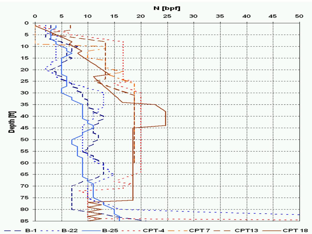
Figure 6 – Composite Plot of In Situ Tests
