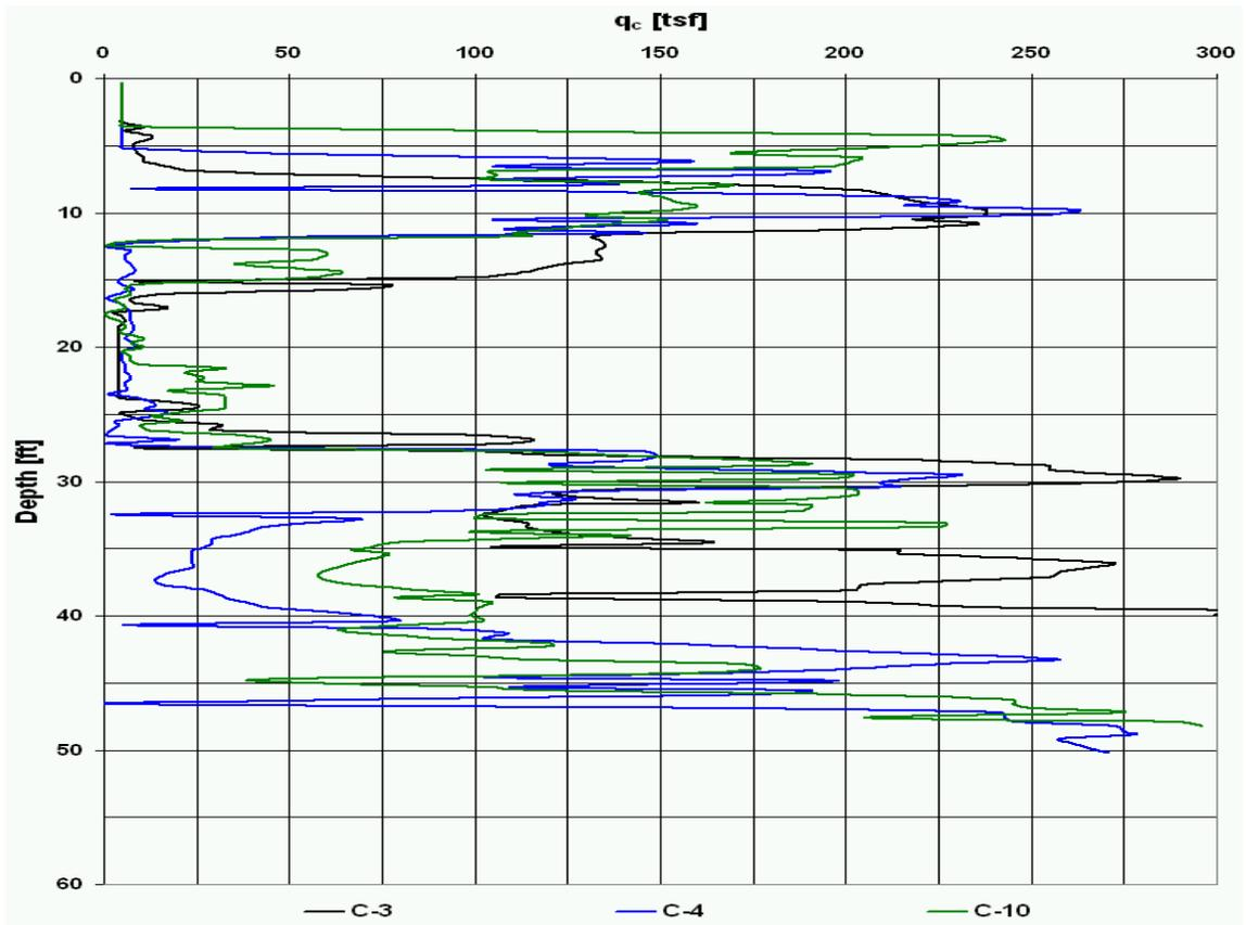
**Figure 9 – Composite Plot of CPT Results**
