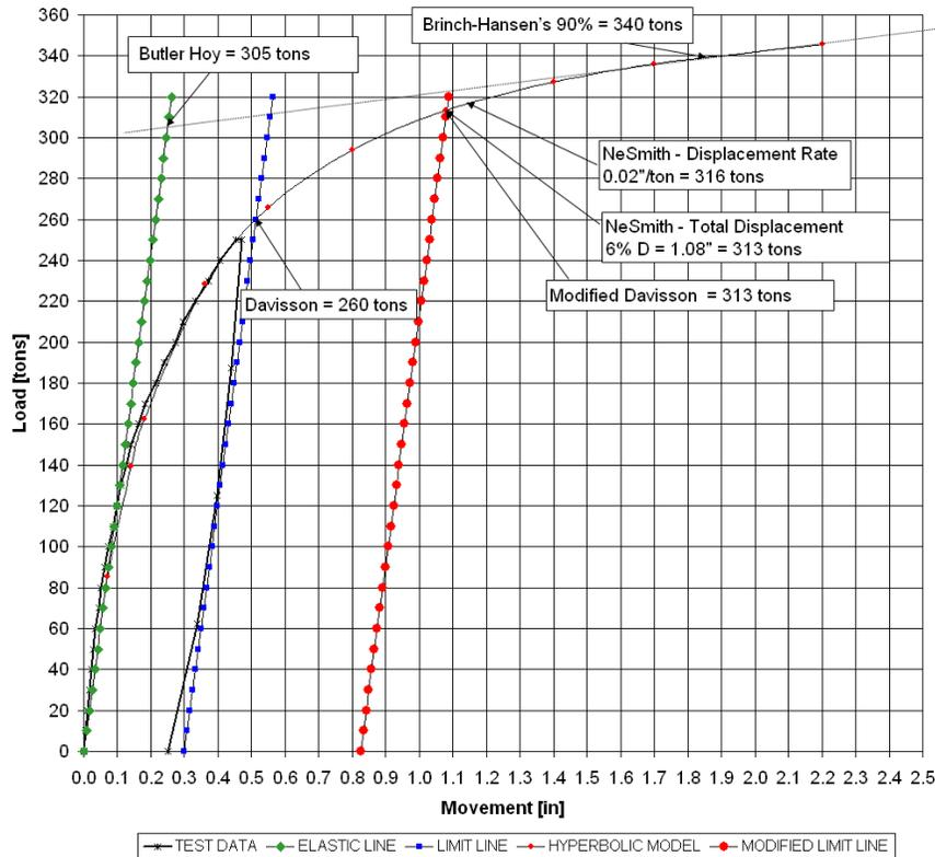
**Figure 8 – Applied Load vs. Pile Head Displacement with Ultimate Load Evaluations**
