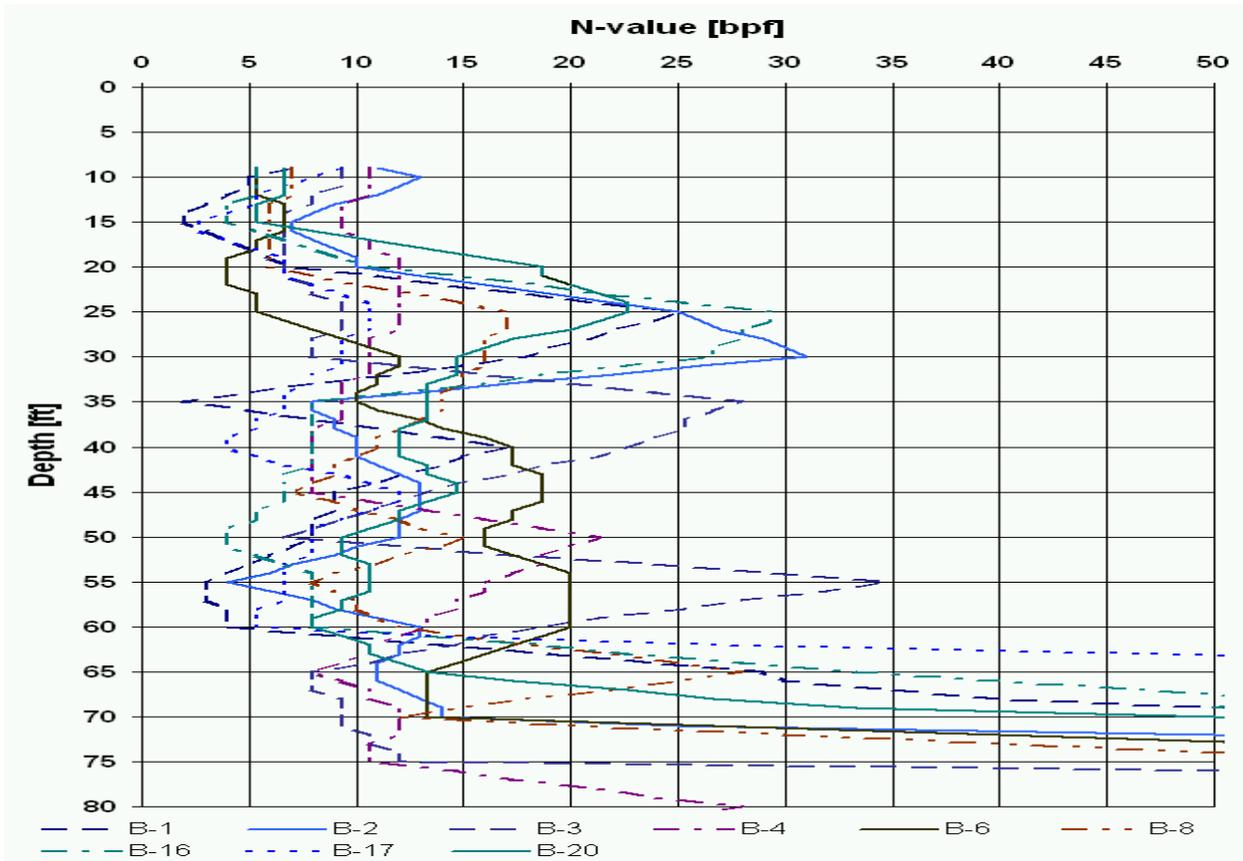
**Figure 11 – Composite Plot of SPT Results**
