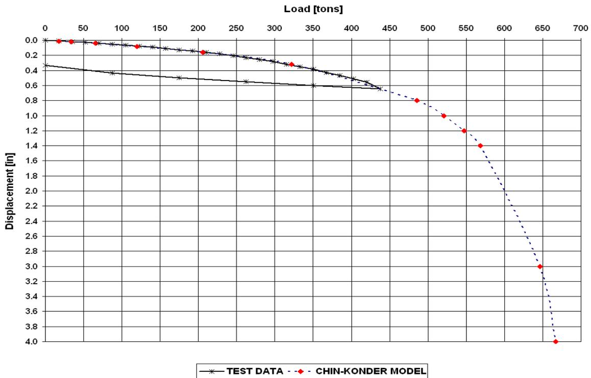
**Figure 15 – Applied Load vs. Pile Head Displacement**
