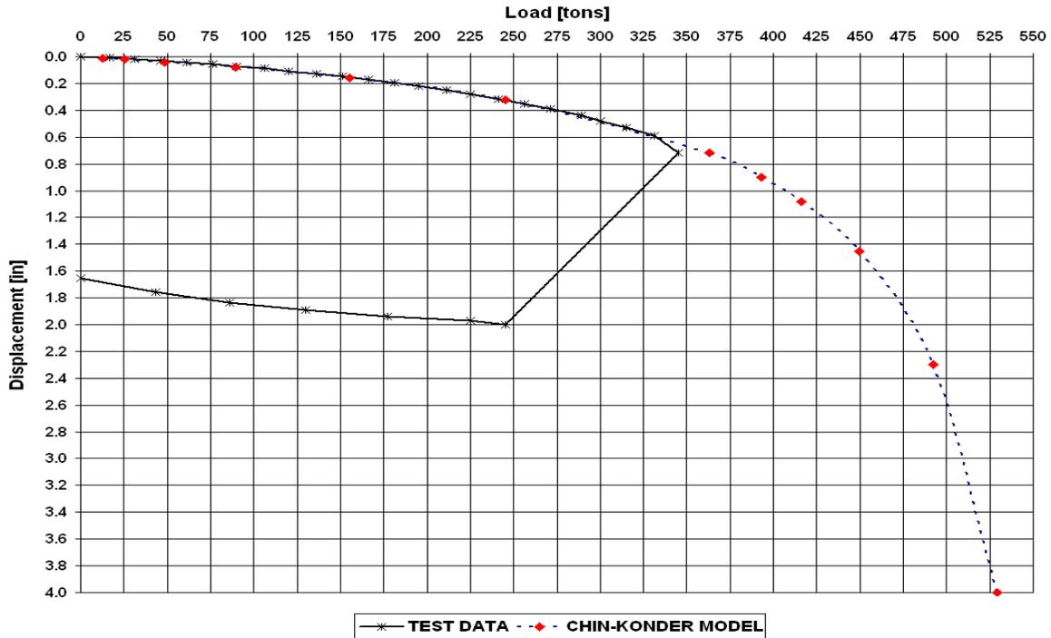
**Figure 13 – Applied Load vs. Pile Head Displacement**
