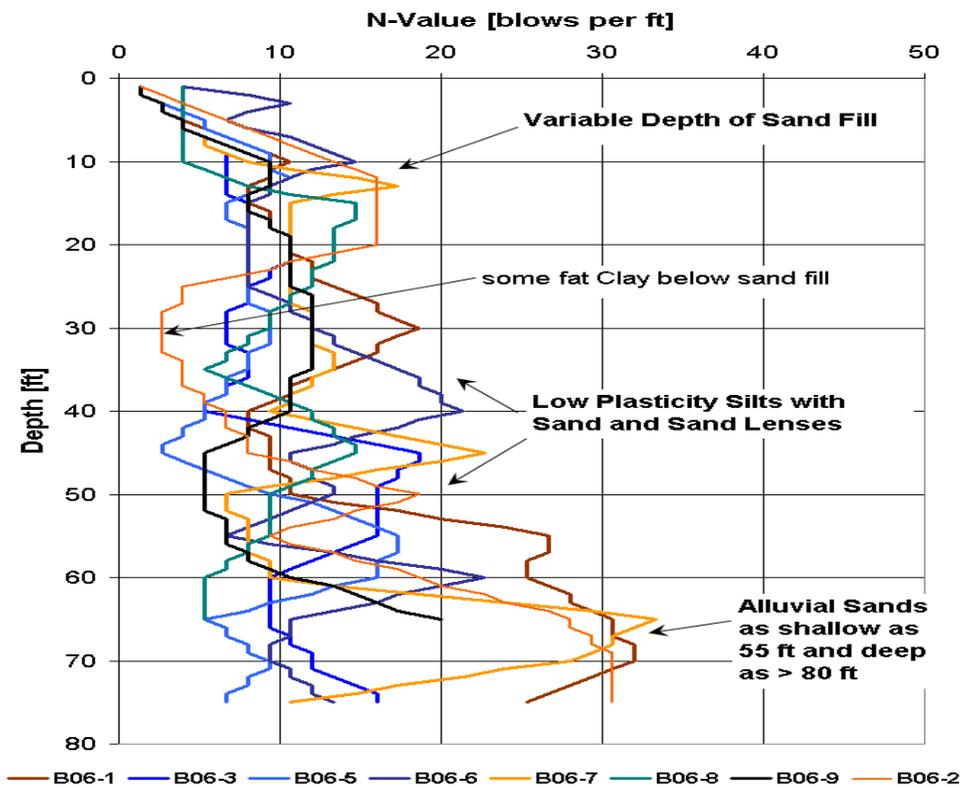
**Figure 16 – Composite Plot of SPT Results**
