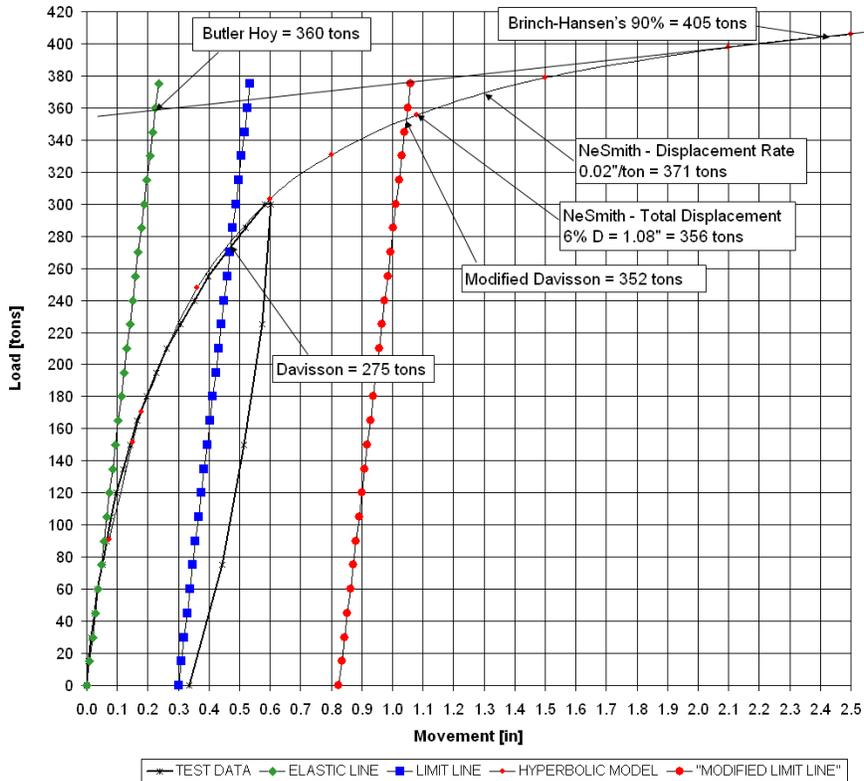
**Figure 7 – Applied Loads vs. Pile Head Displacement with Ultimate Load Evaluations**
