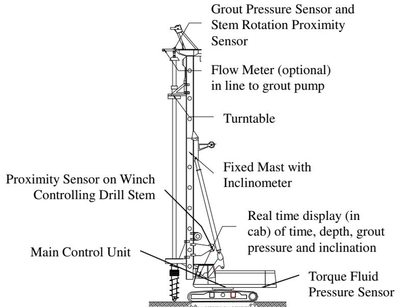
**Figure 1.** Generalization of DAS for Berkel's DD pile drilling platform
