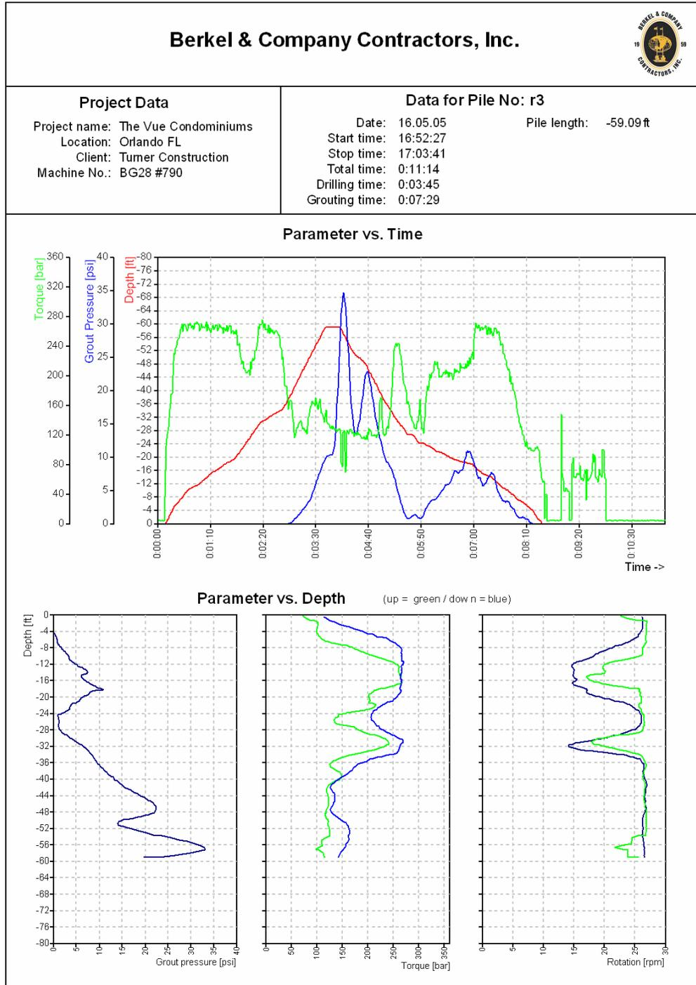
**Figure 6.** Example Plot of DD Pile Installation Data
