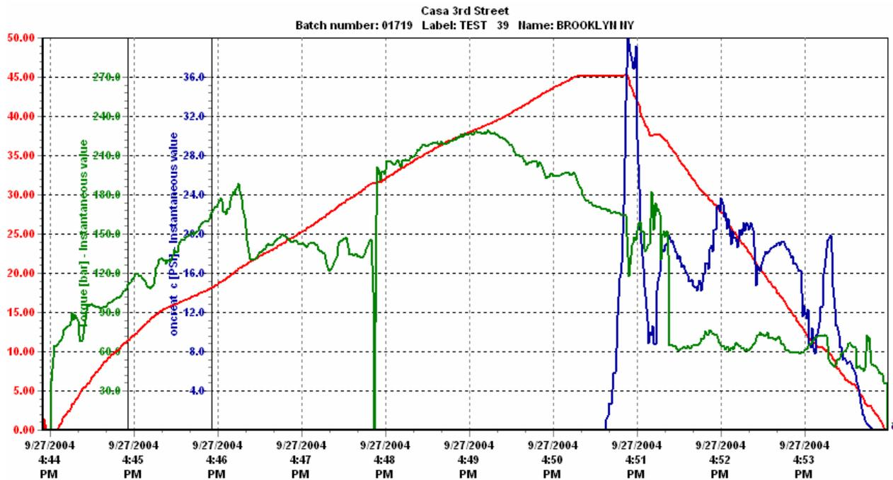
Figure 5. Example Plot of DD Pile Installation Data
