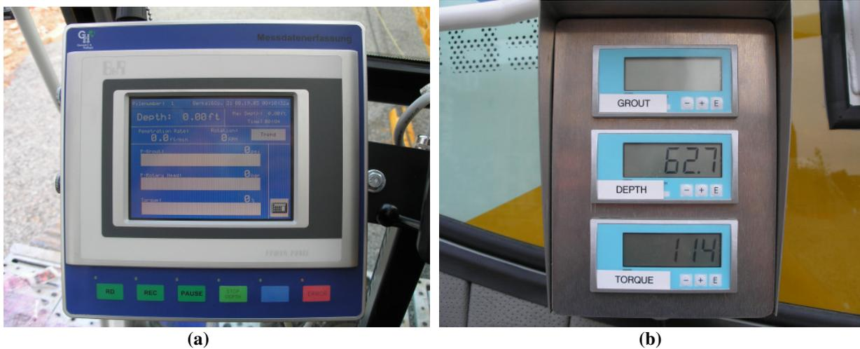
**Figure 4.** (a) real-time graphical display of drilling and grouting parameters in control cabin
