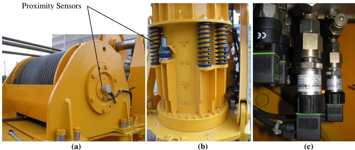
**Figure 3.** (a) proximity sensor on main winch to monitor drill stem depth through main winch rotation
